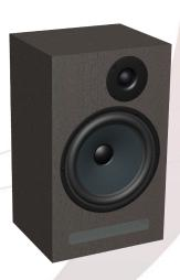
The SEAS A26 is a 2-way loudspeaker kit, using a 26 cm paper cone woofer and a 35 mm textile dome tweeter, in a compact 28 liter aperiodic enclosure. Carefully designed drivers with complementary response characteristics allow for a crossover network using only two components.
